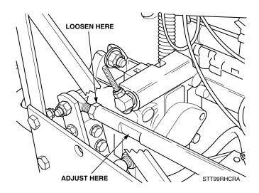
Figure 6-3. RH Steering Control Rod Adjustment
